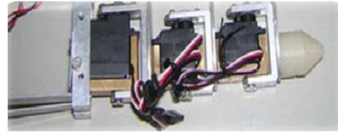
Figure 2. Structures of a fish robot with 4 pieces and 3 links
