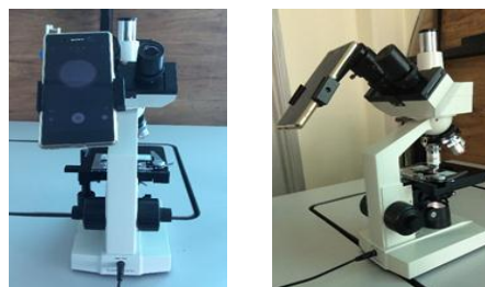
Figure 2. Smartphone attached on the light microscopes
