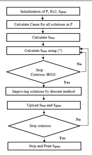
Figure 5. Flowchart of the proposed algorithm (PeSOA\_FSSP)
