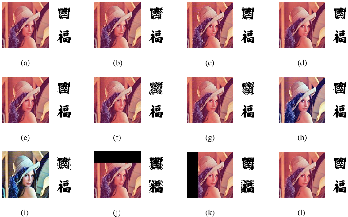
Figure 5. Results under different types of attack and the corresponding recovered watermark using (a) gaussian low pass filter [33], (b) gaussian noise 0.001, (c) sharpening, (d) median filter (3×3), (e) pepper and salt noise 0.1%, (f) speckle noise 0.01, (g) poisson noise, (h) adjust, (i) histogram equalization attack (j) cropping rows off 25%, (k) cropping columns off 25%, (l) scaling 0.5
