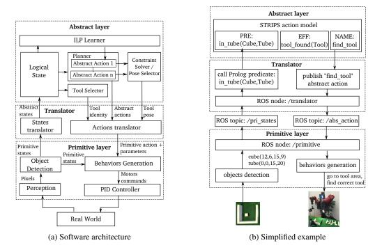
Figure 1. Robot software architecture and its example
