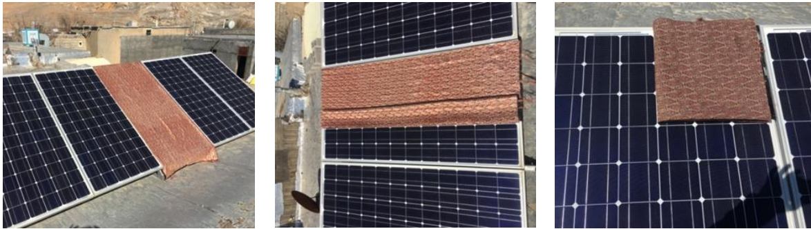
(a) A full panel (b) Two third of a panels (c) One-eighth of a panels
