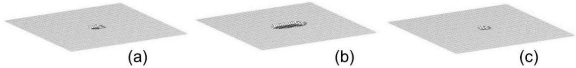
Figure 7. (a) Actual crack, (b) apparent crack deduced from raw image, and (c) inferred crack according to the proposed methodology for Case 3.
