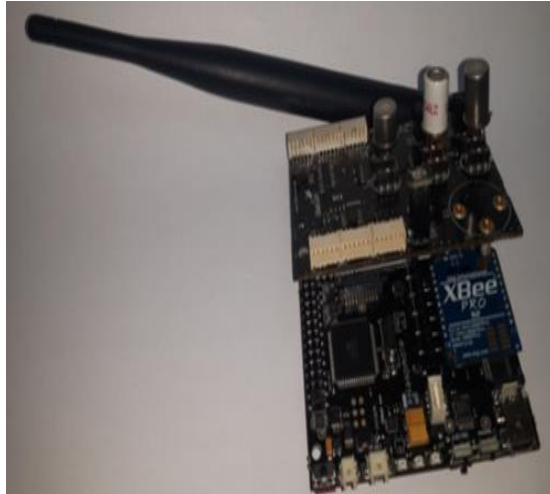
Figure 1. Node integrating the gas sensor board and the XBee antenna
