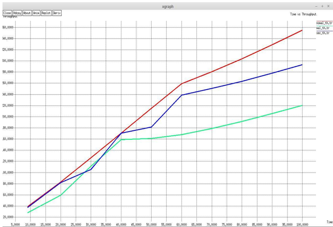
Figure 5. Time vs. throughput curve. nomal_th: Throughput with no malicious node, mal_th: Throughput with malicious node, sec_th: Throughput with security
