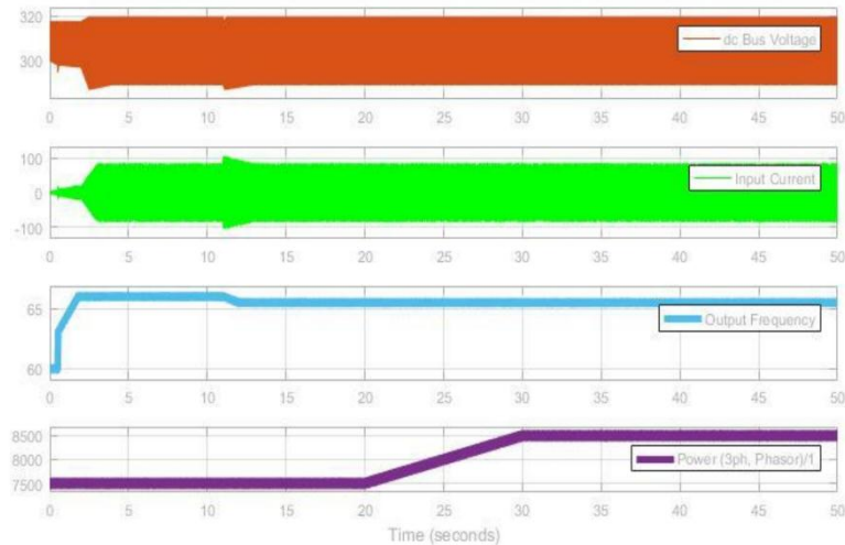
Figure 4. Test results for the dc bus voltage ripple-based frequency fold-back process [15]. Time scale 5sec/div
