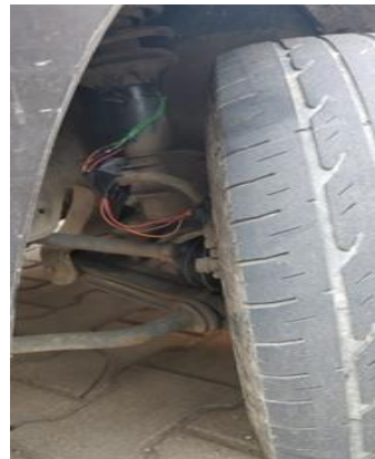
Figure 4. Sensor assembly in the vehicle axle
