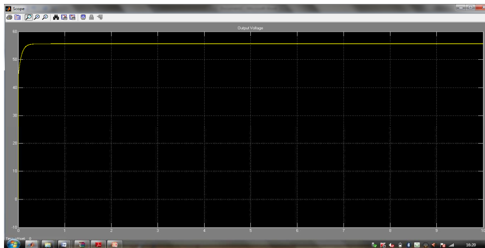
Figure .6 Output Voltage waveform of Boost Converter
