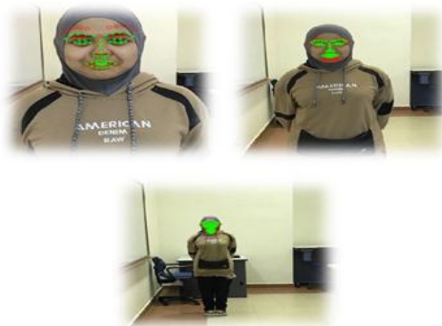
Figure 6. Experiment setup to determine the HR value with detected facial landmarks from distance of 1m (top left), 2m (top right) and 5m (bottom)
