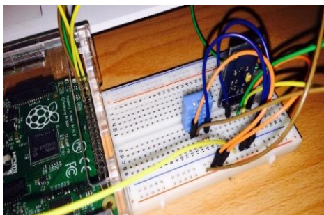
Figure 4. A Raspberry Pi B+ device (left) equipped with sensors (right)
