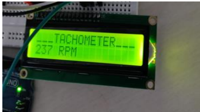
Figure 6. LCD displaying final RPM output
