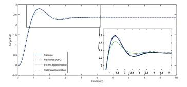
Figure 2. Comparison of step responses of full order model with fractional SOPDT, Routh and Pade approximation
