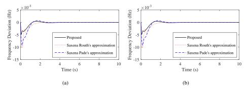
Figure 5. Comparison of response of power system using proposed method with other method for a) lower and b) upper bound uncertainties
