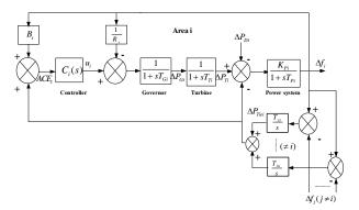
Figure 6. Block diagram of multi area power system
