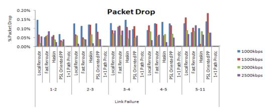
Figure 8. Comparison of packet drop at the five mechanisms
