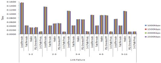
Figure 10. Comparison of the service disruption time in the five mechanisms
