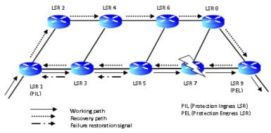
Figure 5. Haskin Recovery Mechanisme [17]
