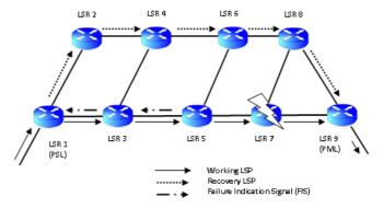
Figure 6. PSL-Oriented Path Protection Mechanisme
