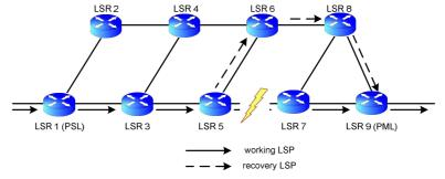
Figure 3. Local Rerouting Mechanisme [17]
