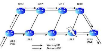
Figure 7. Recovery 1+1 Path protection Mechanism [1]
