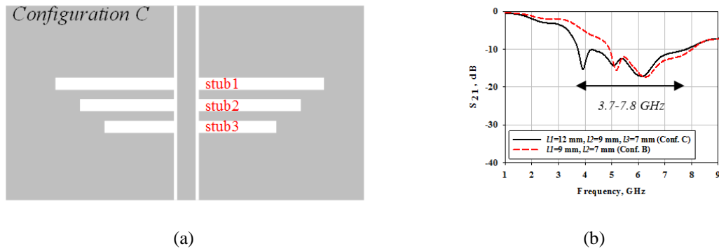
Figure 4. (a) Configuration C - triple-lines, rectangle slot (b) S_{21} result; configuration C vs configuration B
