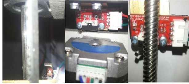
Figure 10. X Y Z limit switches construction
