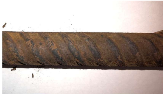
Rebar after corrosion test
