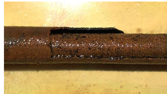
Double tube after penetration
