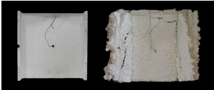
Figure 2.1: Steel profile section protected with a thin intumescent coating, before (left) and after (right) fire testing [18].
