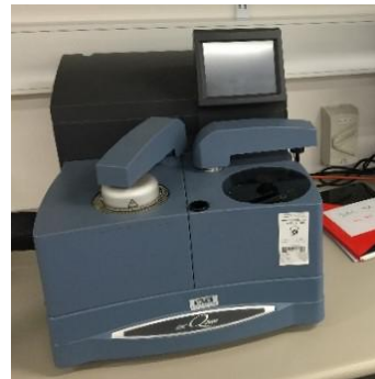
Figure 4.2: Thermal Analysis (TA) Instrument Q2000 for Differential Scanning Calorimetry (DSC).
