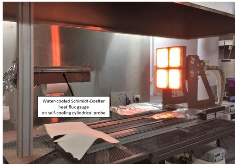
Figure 3.8: H-TRIS calibration procedure ( Bench-scale H-TRIS 2.0 ).
