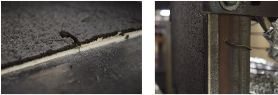
Figure 7.10: Details of the final intumescent char (sample CP-HSC3-01).
