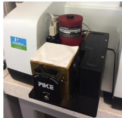
Figure 4.5: Integrating Sphere System (ISS) apparatus (PIKE Upward IntegratIR).
