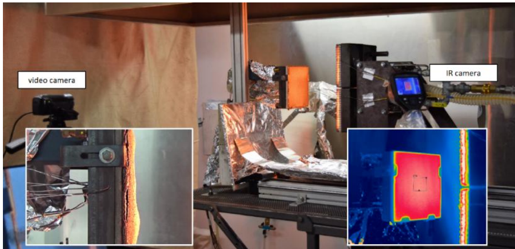
Figure 7.3: Experimental setup designed to gauge the swelled coating thickness and the surface temperature of intumescent coatings during heating exposure ( Sample holder B ).
