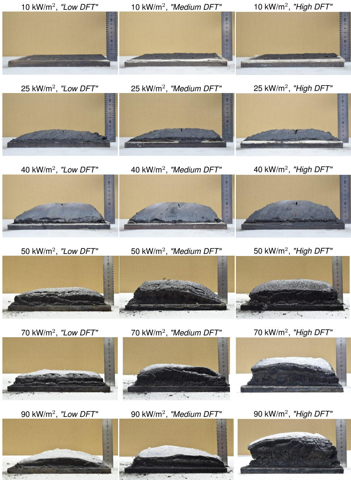
Figure B.2: Comparison between typical porous chars (whole) developed by the intumescent coating at the end of the thermal exposure for different constant incident heat fluxes and applied initial thickness.
