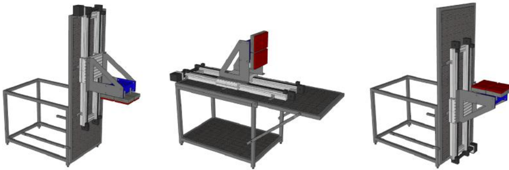
Figure 3.5: Possible experimental configurations of the Bench-scale H-TRIS : vertical configuration with radiant panels array moving downwards (left), horizontal configuration (centre) and vertical configuration with radiant panels array moving upwards (right) ( Bench-scale H-TRIS 2.0 ).
