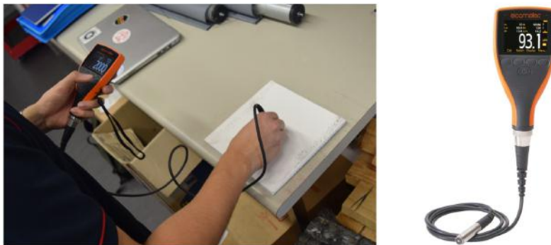
Figure 3.13: Dry film thickness (DFT) measuring procedure using the non-destructive coating thickness gauge Elecometer 456 (device accuracy: \pm 10 \mu\text{m} ).
