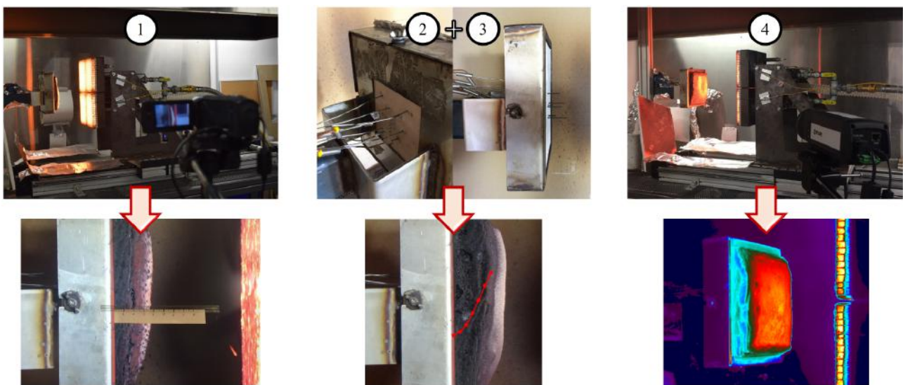
Figure 6.2: Different aspects of the experimental setup designed to gauge the thermo-physical response of intumescent coatings during heating exposure.
