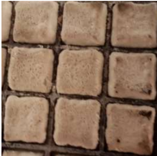
Figure 6.10: Short 3mm fibre reinforced PP post fire testing
