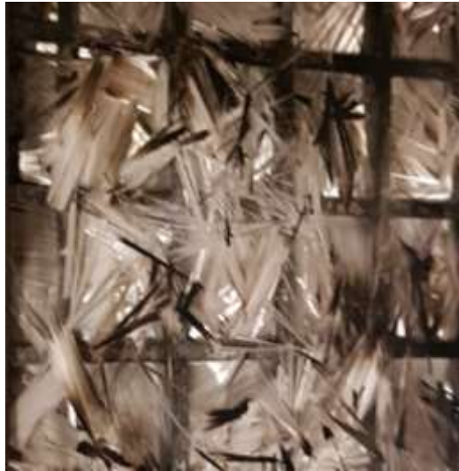
Figure 6.9: Long 12mm fibre reinforced PP post fire testing
