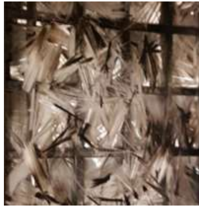
Figure 9.9: Lofting of 12 mm long glass fibres as a result of composite exposure to fire
