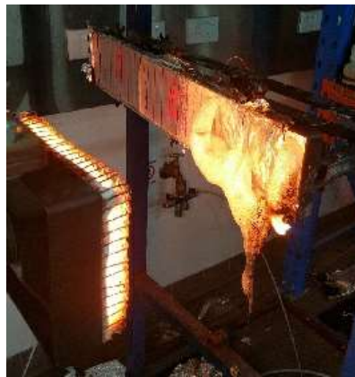
Figure 7.6: A failed attempt of flame spread test for unreinforced PC
