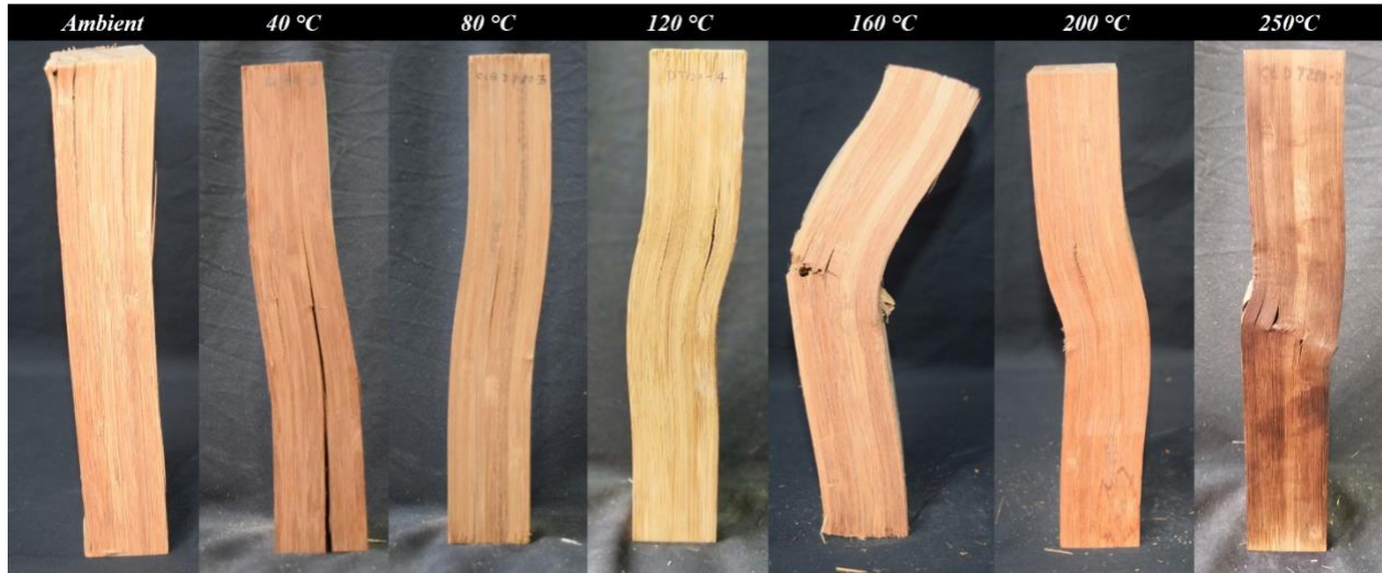
Figure 5. Laminated bamboo failure modes at different temperatures in compression.
