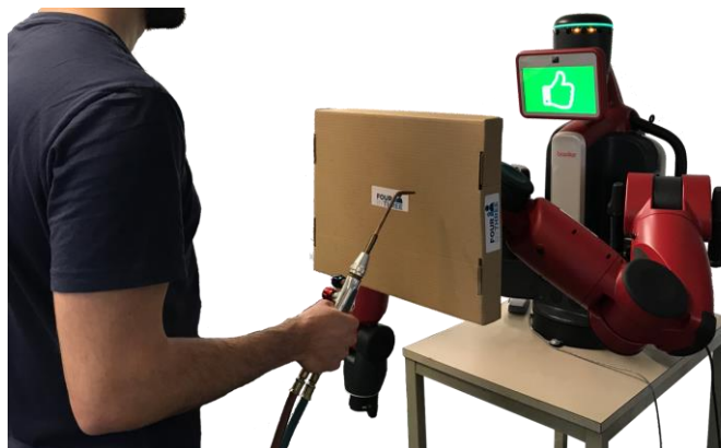
Figure 1 – Robot-assisted ergonomics: the robot monitors the human's ergonomic state in real-time, understands it and optimises the relative pose between the human and the workpiece constantly improving ergonomics.
