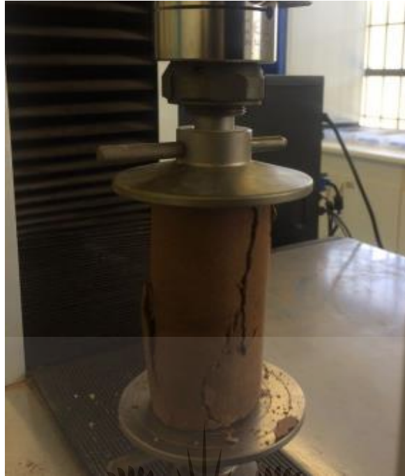
Figure 10.1: Effects of 30% UCS pre-compression stress.
