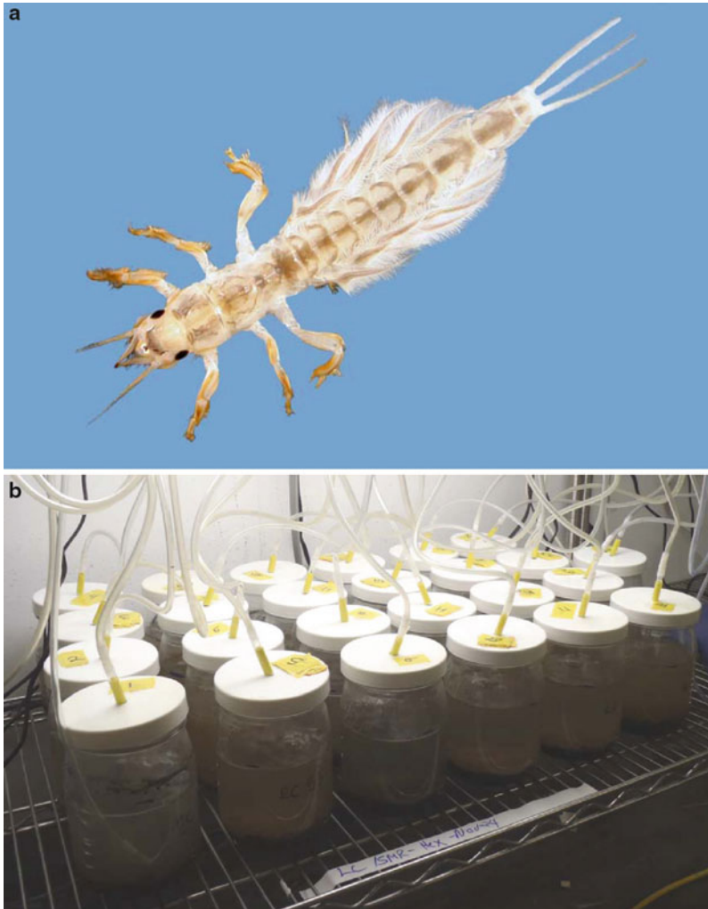
Macroinvertebrate Ecotoxicity Testing (MET), Fig. 3 (a) The mayfly, Hexagenia limbata (Photograph courtesy of D. Milani) (b) An example of sediment toxicity tests conducted in 1-L glass jars with Hexagenia limbata . Duration of the toxicity test is typically 3 weeks under static conditions with constant aeration of the overlying water. In a standard toxicity test, each jar contains 650 mL overlying water, 125 mL sediment, and 10 Hexagenia limbata (1.5–2 months old at test initiation). Tests are conducted in an environmental chamber at 23–25 °C with a photoperiod of 16 h light:8 h dark (Day et al. 1998) (Photograph courtesy of J. Baillargeon)
