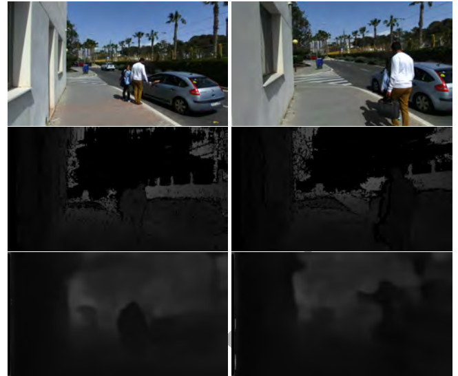
Fig. 14: Results of the depth estimation from monocular frames. First row shows two random samples, second row depicts the corresponding ground truth and third row represent the estimated depthmap as provided by the system. Images are shown for qualitative evaluation only.
