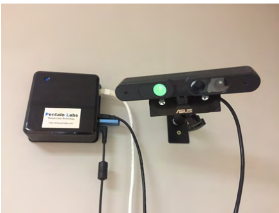
Fig. 1: Asus Xtion camera connected to a small networked NUC computer and installed near to the ceiling and in the corner of a room.
