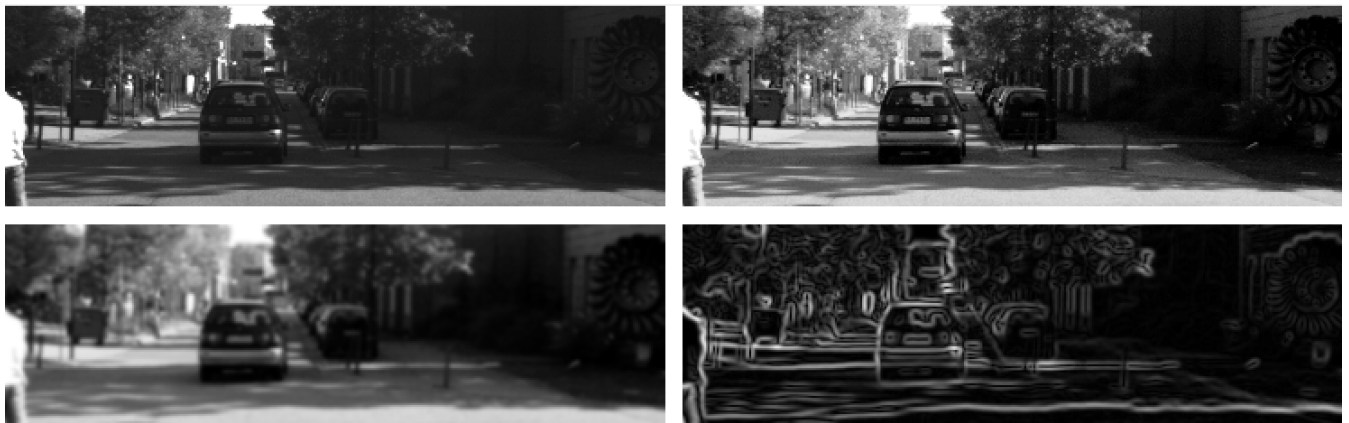
FIGURE 3. Image preprocessing for data readiness for the co-registration stage. Top-left: Original image taken in grayscale. Top-right: Original image after applying histogram equalization. The central part that looked very dark in the original image now shows a higher contrast. Bottom-left: Result of applying a Gaussian filter to the equalized image. Thanks to this process, the image edges are wider so that the alignment is not too restrictive. Bottom-right: Final result of the process that provides the image \mathbf{E} . For this process, we apply the Sobel gradient operator in order to obtain the edge intensity at each point of the image.
