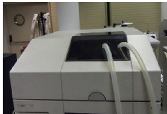
Fig. 1. (A) Mini-thermostatic device (MTD). (B) Cassette and front cover of the Agilent HP3DCE instrument with the home-made high performance thermostatzation system installed on it.
