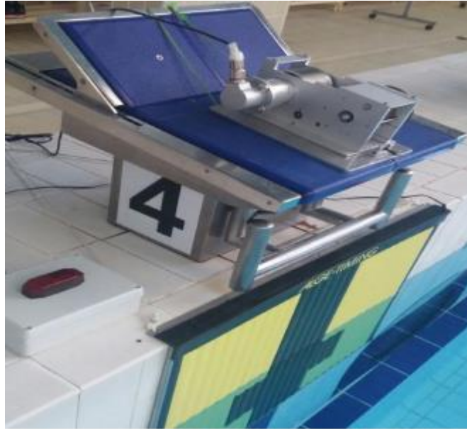
Figure 4. Speedometer used for the measured of the instantaneous swimming velocity (lineal transducer, Heidenhain, D83301, Traunreut, Germany).
