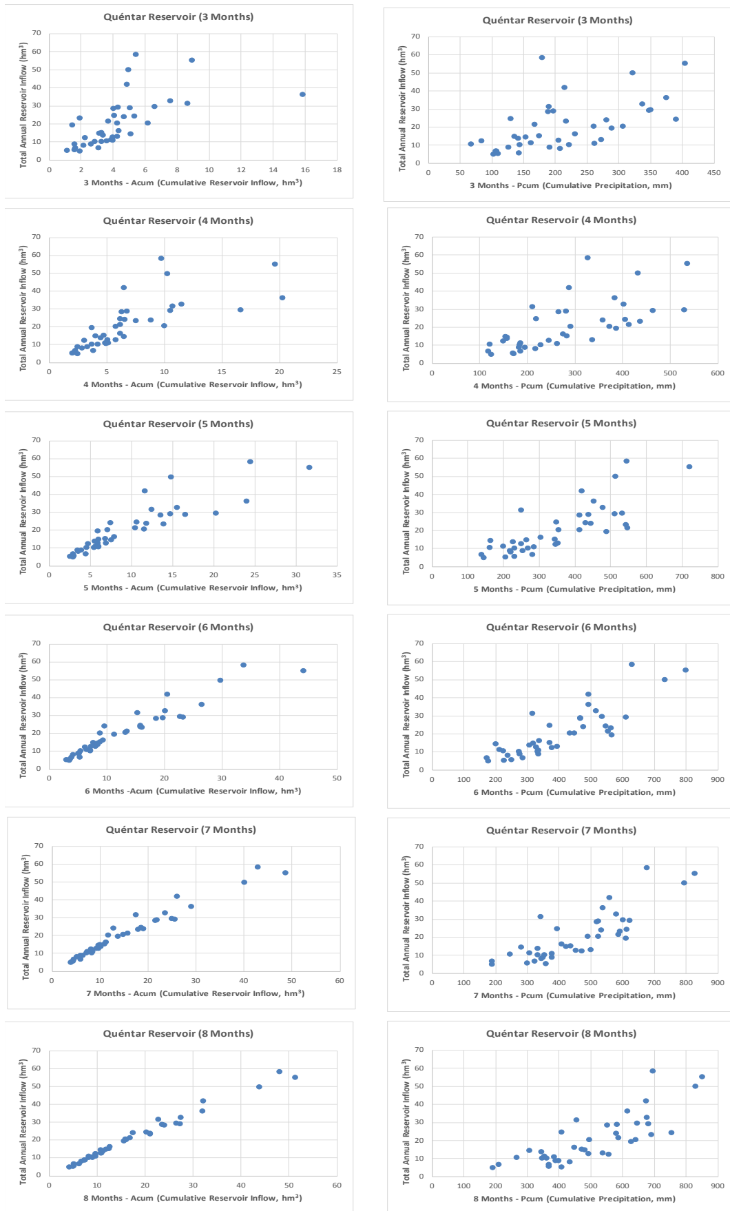
Figure 26: Quéntar reservoir: Regression analysis for the first three, four, five, six, seven, and eight months using the cumulative monthly reservoir inflow and precipitation (power model regression).
