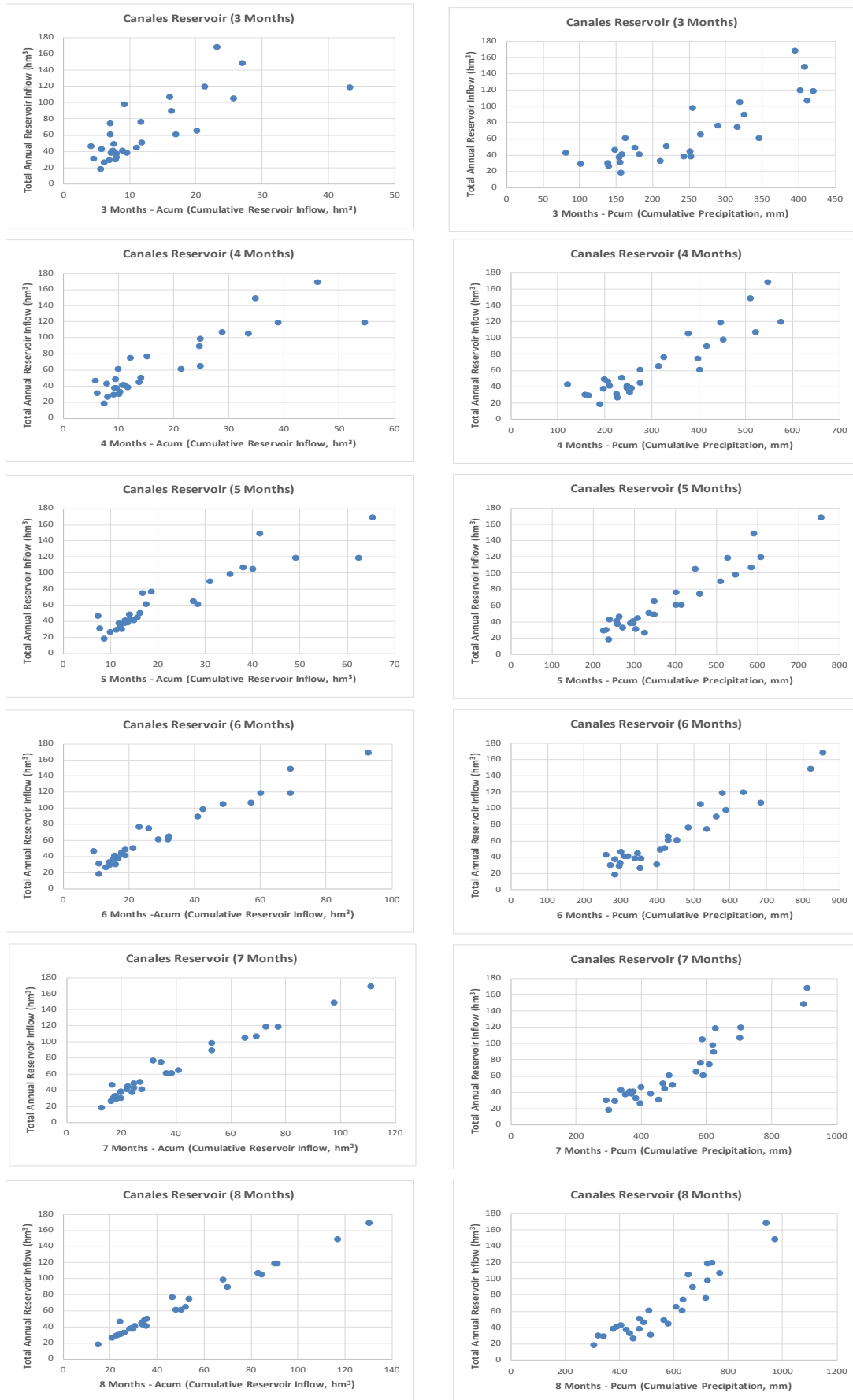
Figure 25: Canales reservoir: Regression analysis for the first three, four, five, six, seven, and eight months using the cumulative monthly reservoir inflow and precipitation (linear model regression).
