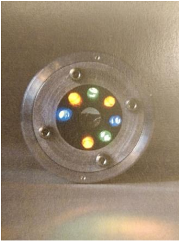
Figure 3. The LED's equipped on BenthosTorch. The "empty" spot indicates the location of the additional LED (wavelength 700nm). The wavelengths are 470nm (=blue), 525nm (=green) and 610nm (=yellow; bbe-Moldaenke, 2014).
