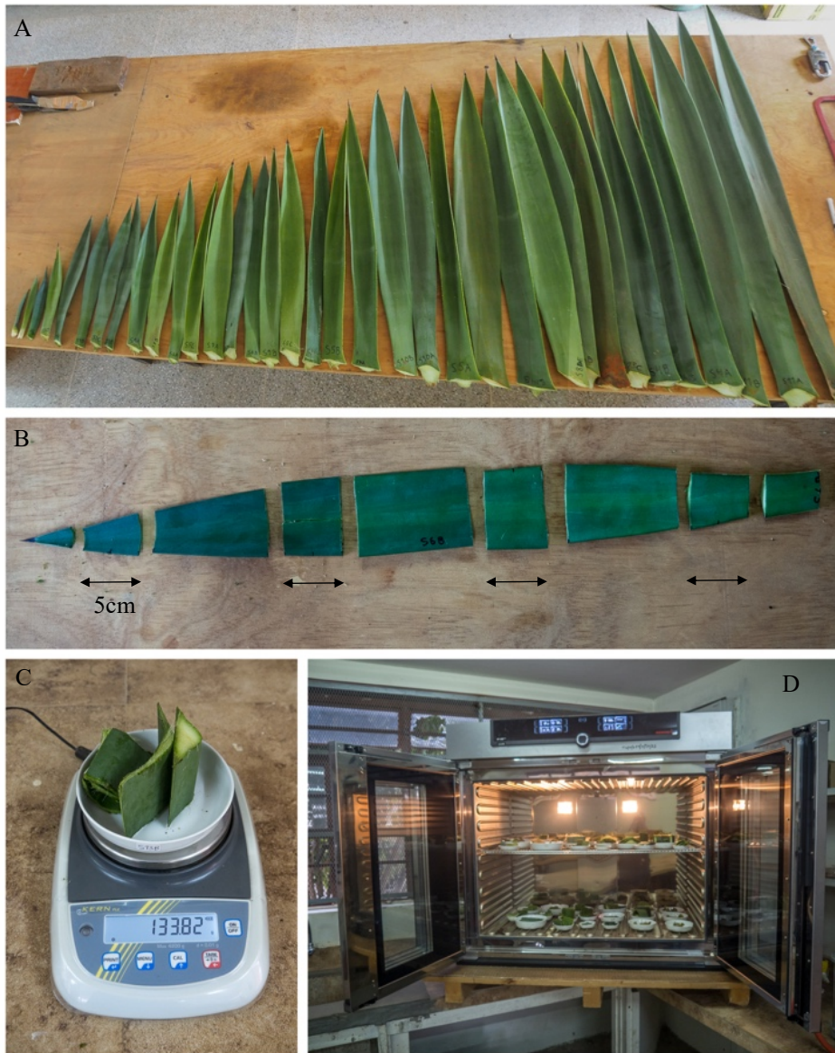
Fig. 9. Measuring leaves for allometric modelling. (A) The whole leaf sample. (B) Sub-sampling a leaf for drying. (C) Sub-sample weighing. (D) Subsamples placed in the oven for drying.
