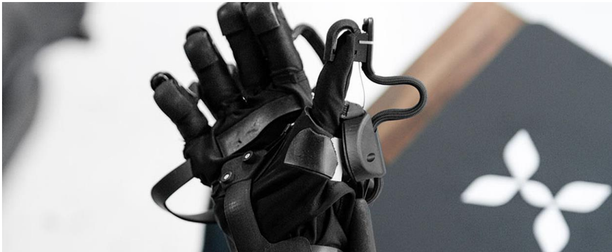
Figure 2. HaptX Glove that provides finger tracking as well as haptic feedback (Source: Nordrum, 2017)
