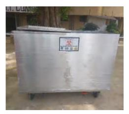
Figure 5.19 Transport trolley for healthcare waste (Source: UNIDO 2018:55)
