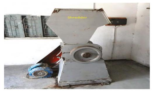
Figure 5.32 Shredder (Source: UNIDO 2018:92)
