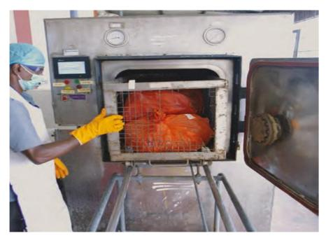
Figure 5.24 Autoclave (Source: UNIDO 2018:89)
