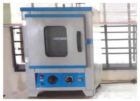
Figure 5.25 Circulating hot-air oven (Source: UNIDO 2018:89)
