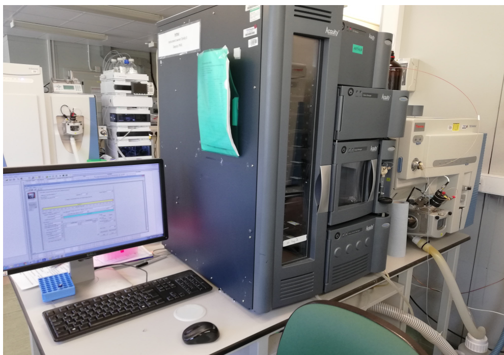
Figure 3.3: (A) Simple schematic for LC-MS and (B) Photograph of the set-up, showing Thermo Xcalibur software and automated injection port.
