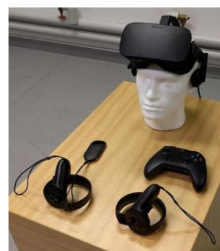
Figure 2. The Oculus Rift HMD with its interaction devices including wireless hand controllers
