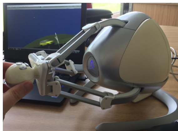
Figure 3: The Novint Falcon being used to control a virtual needle in ParaVR
