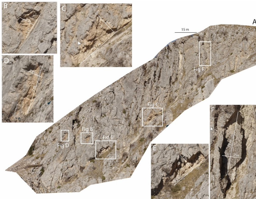
Figure 17. The 3D model of the area UAV 2 (A), examples of rockfall scars (B–E) and a suspended block (F). The calculated volume of failed blocks associated with such scars is ca. 40 m 3 (Figure 17B), ca. 200 m 3 (Figure 17C), ca. 60 m 3 (Figure 17D) and ca. 230 m 3 (Figure 17E). Figure 17F highlights the volume of overhanging block with a volume of ca. 500 m 3 .
