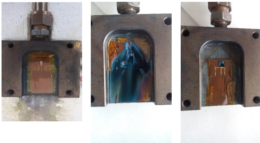
Fig. 4.11 AA-CVD deposition steps.
