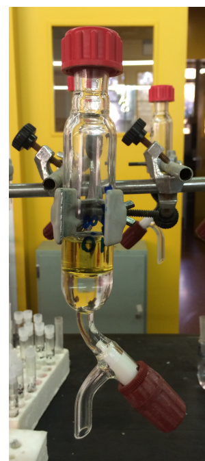
Figure 27. Separatory funnel used for LLE.
