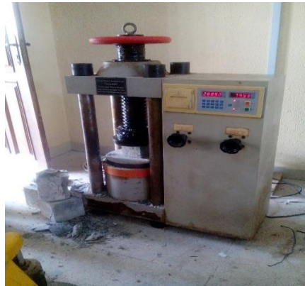
Fig. 1. Compression machine use for both compressive and split tensile strength tests with cube under load.
