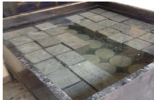
Figure 2. Samples placed in the curing pond
