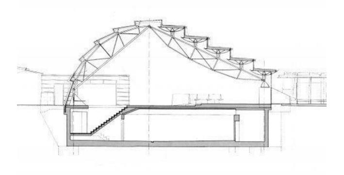
Figure 4. 3: Section of the Nil Ericson terminal, showing the large hall and the basement garage Source: Lindstrom (2013)
