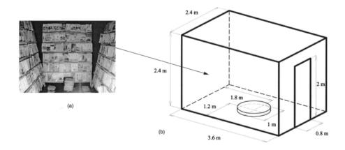
Figure 2. 15: This is the newspaper shop and its geometry where the fire test was performed. *Source:* Chow (2005)
