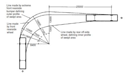
Figure 2. 8: Shows a 10 m bus making a turn of 90 degrees Source: Blow (2005)
