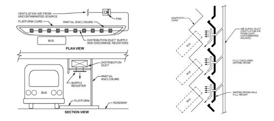
Figure 2. 14: On the left side is a drive-through with semi-enclosed platform, on the right is a fully enclosed waiting room with sawtooth gates.
