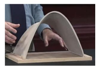
Plate 3. 11: View of the parabolic shape on the hyperbolic paraboloid Source: Ressler (2017)
