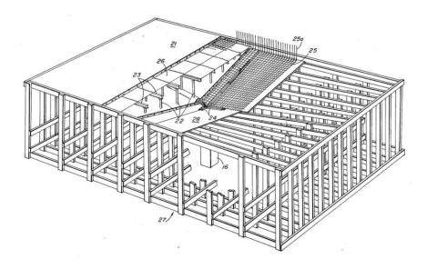
Figure 3. 4: Perspective partial cutaway view of several layers of forms and reinforcement materials usable in hyper umbrella
