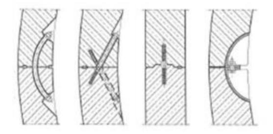
Figure 3. 7: Bolt connection joint in concrete Source: Maten (2011)
