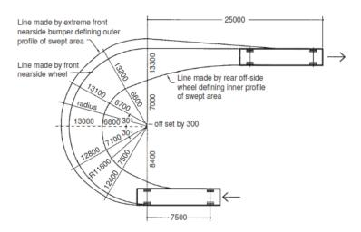
Figure 2. 9: A bus of length 12 m making a turn of 180 degrees Source: Blow (2005)
