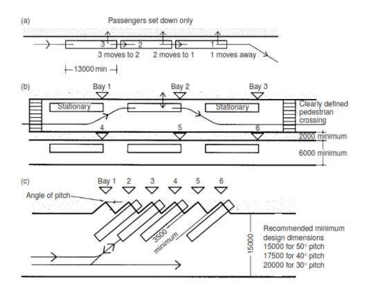
Figure 2. 11: The way buses approach platforms a) shunting, b) drive-through c) sawtooth Source: Blow (2005)
