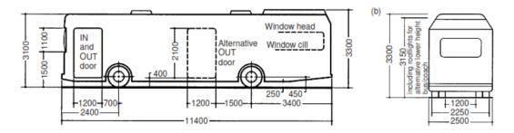
Figure 2. 7: Typical length and width of a bus Source: Blow (2005)
