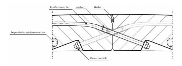
Figure 3. 8: Detailed connection between thin-shell prefab elements using bolted connection Source: Maten (2011)
