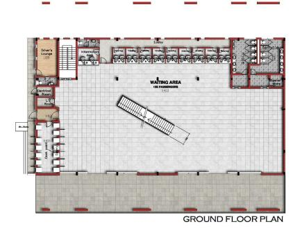
Figure 4. 25: Ground floor of Ikeja bus terminal building Source: Plant Project Limited (2018)
