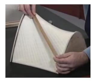
Plate 3. 12: Ruler laid flat on the surface of hyperbolic paraboloid Source: Ressler (2017)
