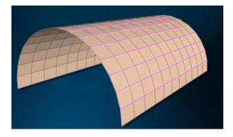
Plate 3. 3: Cylinders have curvature in one direction only Source: Ressler (2017)
