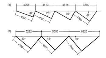
Figure 2. 12: Dimension and angles in sawtooth configuration Source: Blow (2005)
