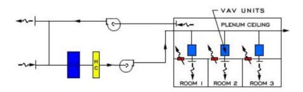
Figure 2. 13: All-Air central system diagram of the category variable air volume (VAV) Source: Commercial Energy Library (2013)
