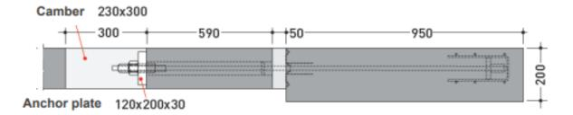
Figure 3. 9: Section of fixation of precast element to existing structure using post-tension connection Source: Maten (2011)
