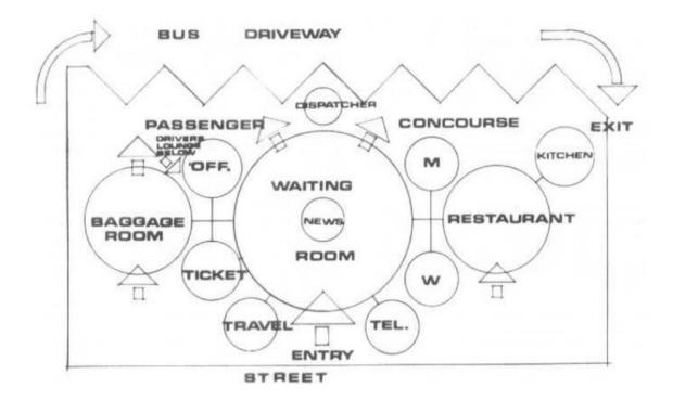
Figure 2. 5: Flow diagram Source: Chiara (1990)
