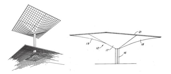
Figure 3. 2: On the left is the hyper umbrella on its foundation and on the right is its frontal view Source: Tully (1979)
