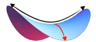
Plate 3. 14: The red arrow represents compression and the black arrow represent tension Source: Bhatia (2014)
