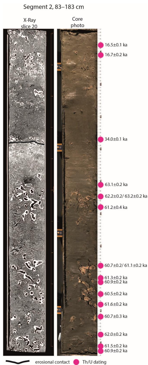
555 Appendix Figure B: CT image (left) and photography (right) of segment 83-183 cm of core M125-34-2. Erosional contacts are marked by thick black lines, position of Th/U datings with calibrated ages are indicated by magenta dots.
