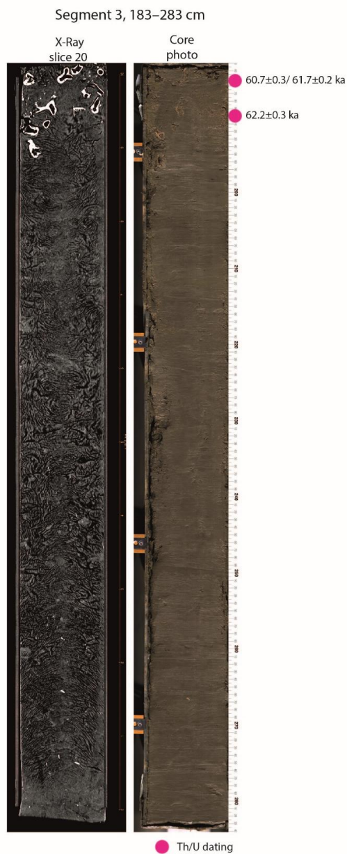
Appendix Figure C: CT image (left) and photography (right) of segment 183–283 cm of core M125-34-2. Position of Th/U dating with calibrated age is indicated by a magenta dot.
