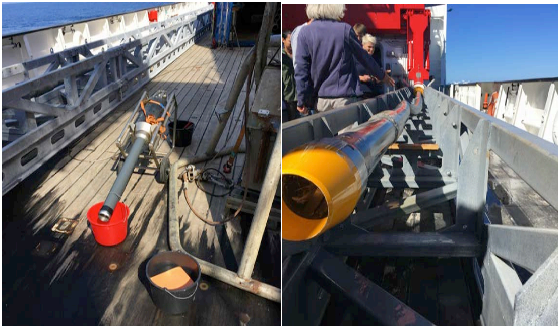
Pilot core of piston coring system. Gravity corer after retrieval with insufficient penetration resulting in bent core barrel ("banana")
