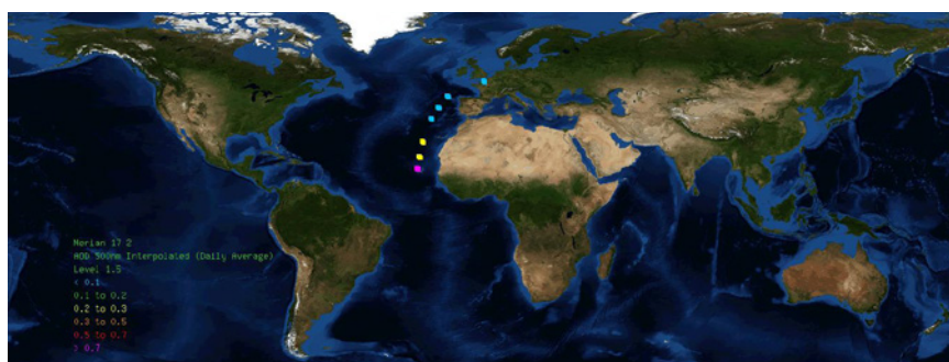
Fig. 2: Measurements of the aerosol optical depth from MSM 68/2. Larger values (yellow and pink) mark the occurrence of dust aerosols from North Africa.
