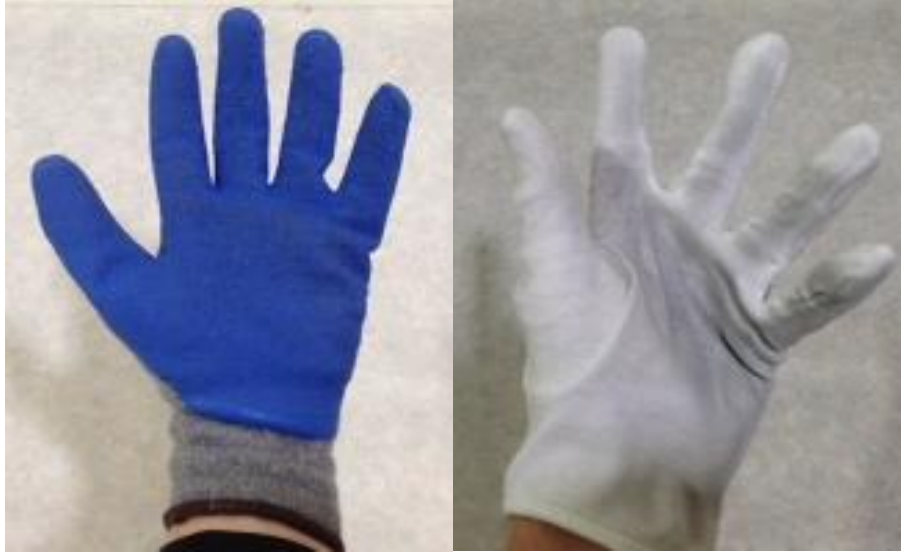
Appendix Figure 30: High friction and low friction glove condition. The high friction glove (left) is made of knitted fabric with a latex palm and the low friction glove (right) is made of 100% cotton.
