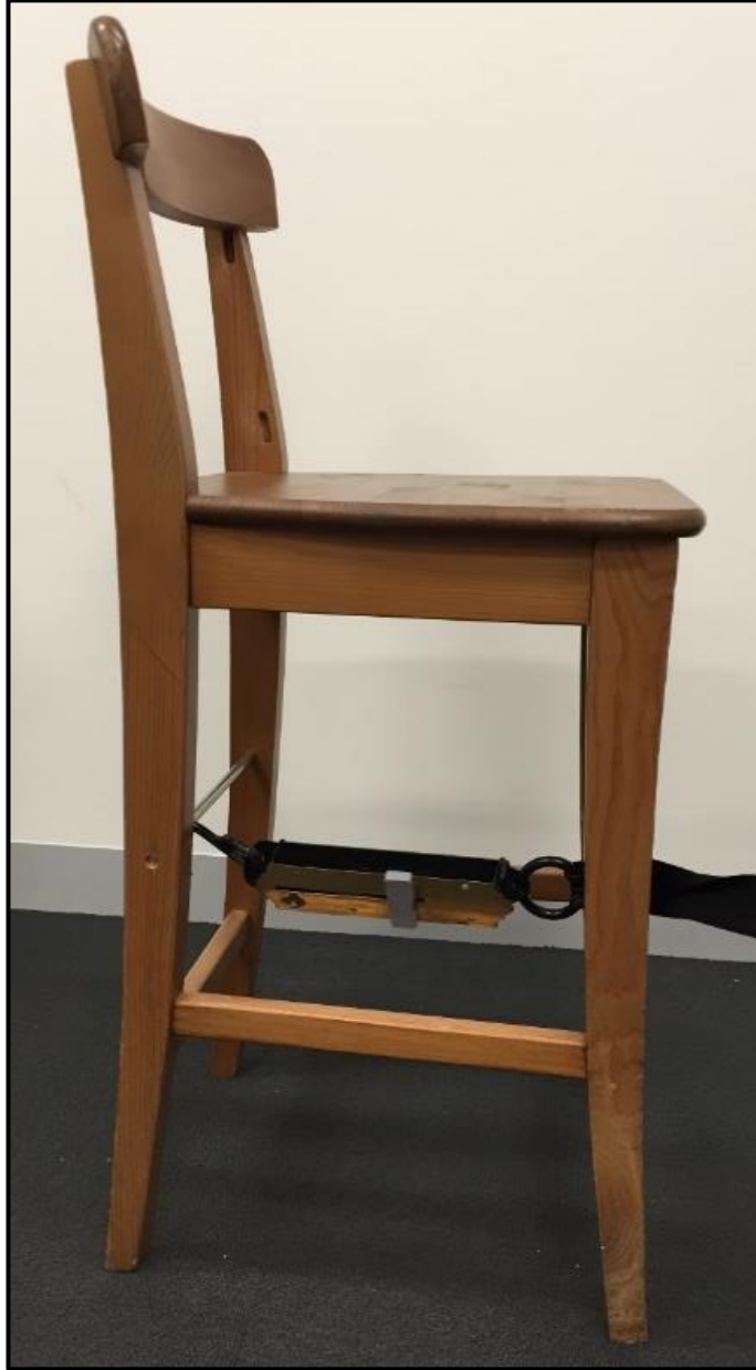
Appendix Figure 16: Knee strength. Participants sit in a high chair. A strap in-line with a scale is secured just above the ankle of the dominant leg. Participants are encouraged to kick their dominant leg out to the best of their ability. The leg is secured, preventing movement, resulting in an isometric knee extension contraction. The extension force is recorded by the scale. Scoring is based on the maximum knee extension force. A higher score is associated with a greater knee strength.
