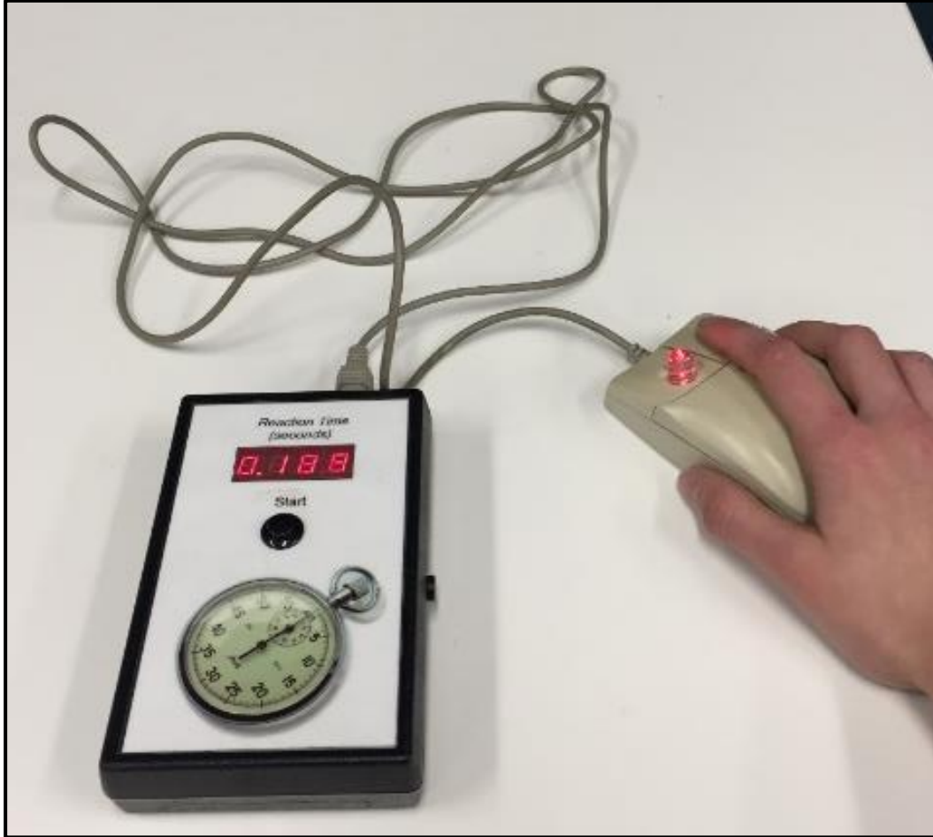
Appendix Figure 14: Hand reaction time. Scoring is based on the average time to left click on a computer mouse in response to the illumination of a red LED. A higher score is associated with a slower reaction time.
