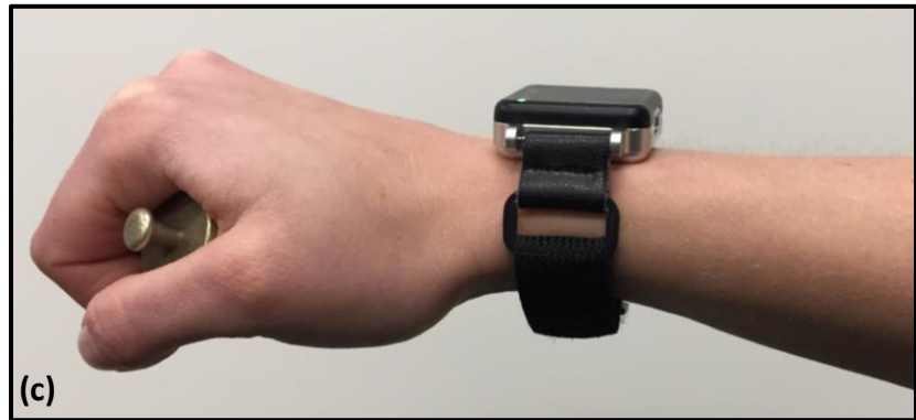
Appendix Figure 10: Arm stability. Scoring is based on the total path length traveled that was recorded from an IMU on the wrist when holding the outreached dominant arm as straight as possible for 30 seconds. Participants completed this task with a closed fist and eyes open (a) and with 250 grams (b) inside a closed fist with eyes closed (c). A higher score is associated with reduced arm stability.
