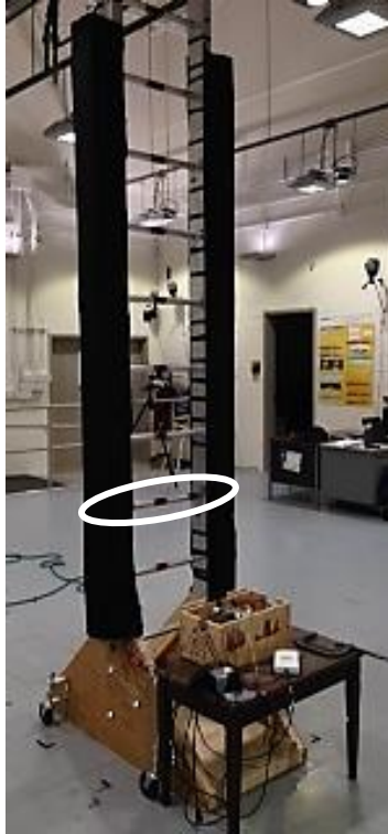
Figure 4.1.1: Instrumented ladder. The ellipse encircles the electronically-controlled releasing rung.
