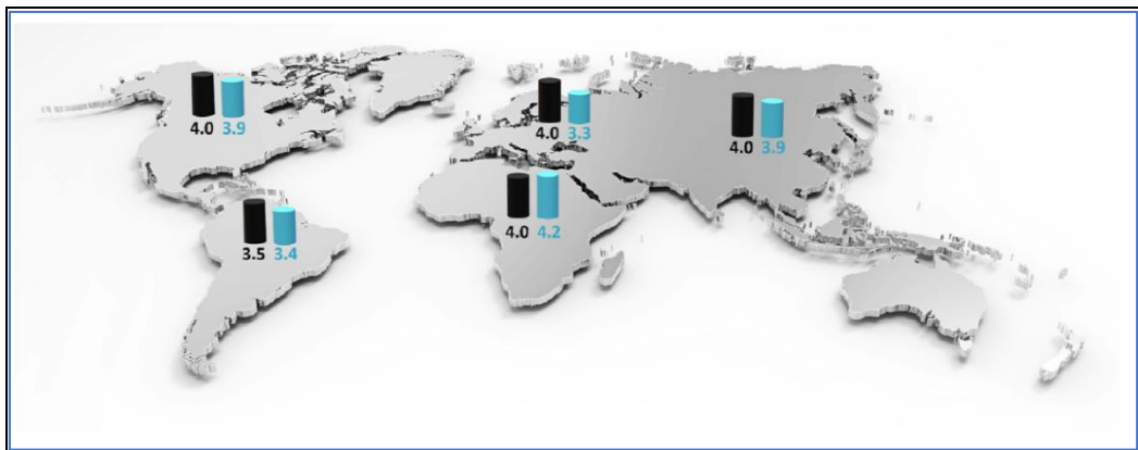
Figure 7. Equivalent inertia constants are estimated worldwide for each continent. Change between 1996 and 2016 [6]
