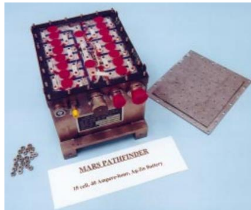
Figure 2. Mars Pathfinder. Silver-Zinc Battery. (Photo courtesy of Jet Propulsion Lab.) [9]
