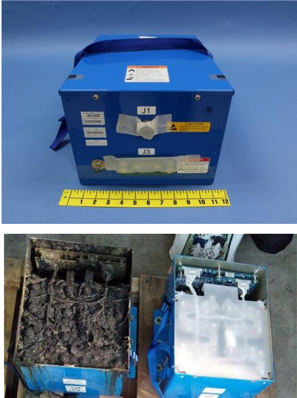
Figure 1. Fire of the Li-ion battery [3]
